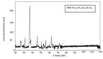
Fig 1.1: X-ray diffraction photograph of Li 0.5 Fe 0.5+x Al12-2xCoxO19
