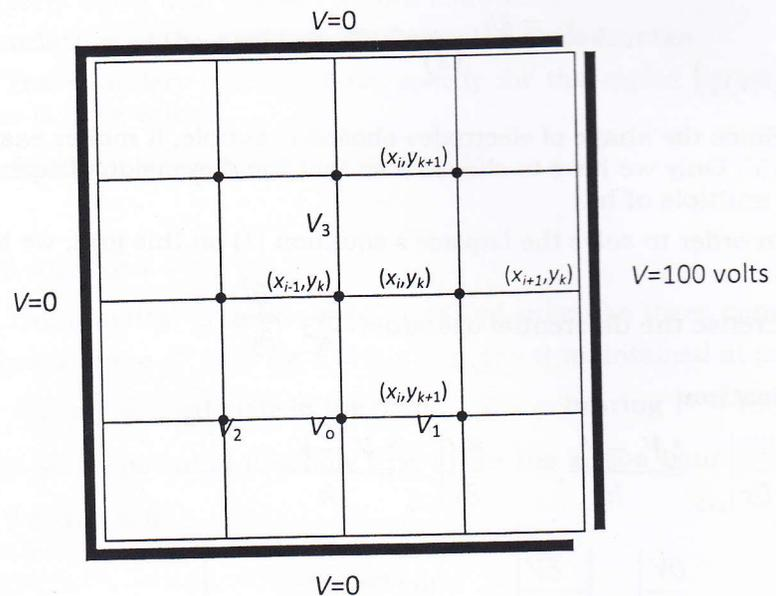
**Fig.2** Calculation of potential by approximation formula
