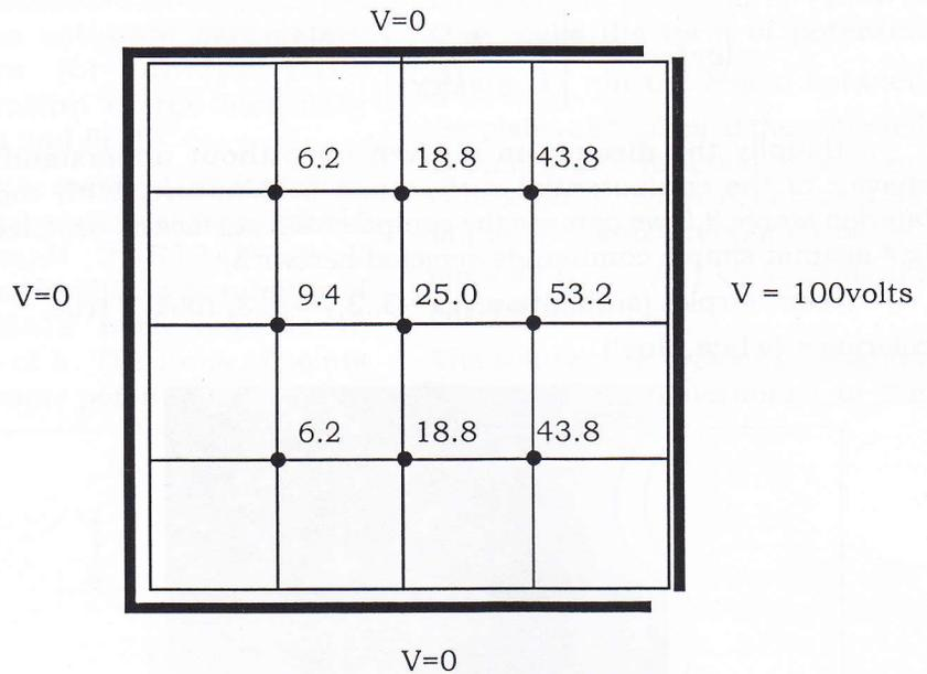
**Fig.3** Calculation of potentials in 16 sub square corners
