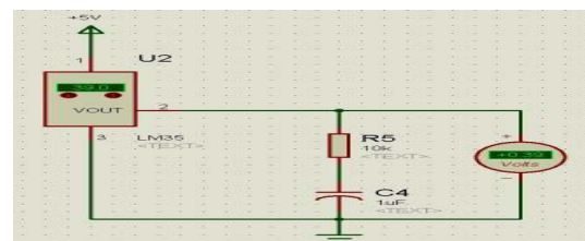
Fig 3. Temperature sensor circuit
