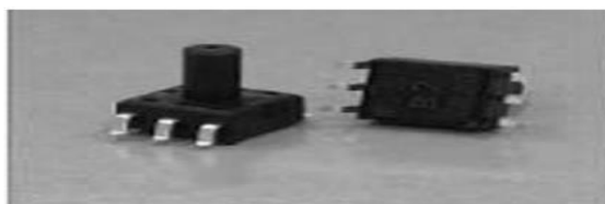
Fig 3.3 Blood pressure sensor MPS-3117
